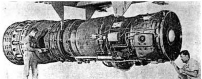
The J58 was later equipped with an after burner. This model was usually presented as a J58-P2 destined to equip the F8U-3 and A3J of the US Navy.
