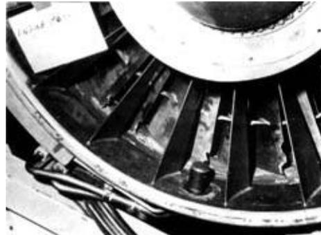
J-58 air inlet after the ingestion of an inspector's flashlight in charge of checking for foreign objects...Total damages: \$ 250,000.
