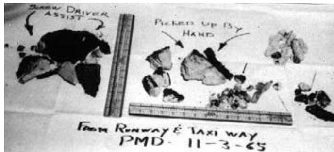
Some examples of foreign objects absorbed by a J-58 during taxi tests: parts of a screwdriver, gravel, chunks of asphalt...
