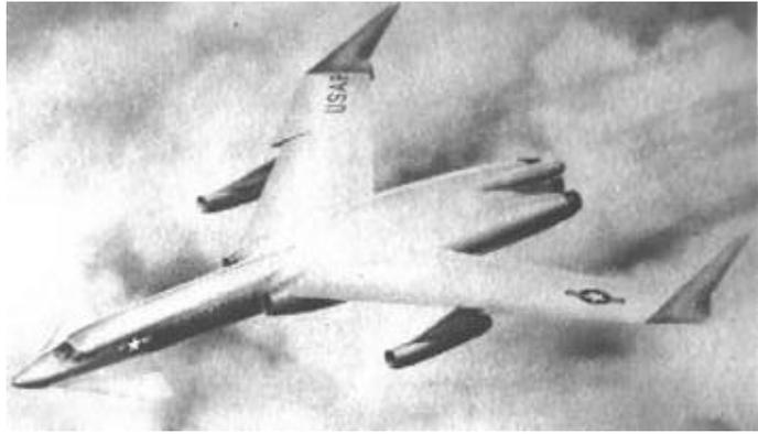
This strange experimental aircraft, the Convair NX-2 was to be built (two of them) to test the General Electric and Pratt & Whitney nuclear engines. Effectively, an atomic version of the J-58 was seriously considered.
