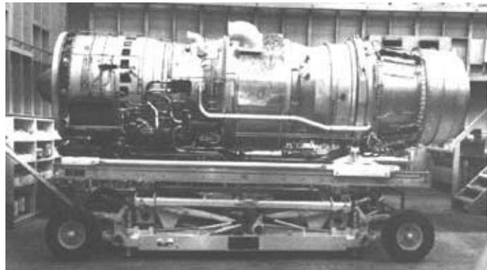
This full-scale model of a J-58P2 was made by Pratt & Whitney in Hartford in July 1961 to study the global size of the engine.
